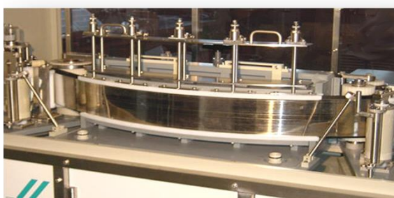
Multiple stripes plating on wide material in using static perforated masking band
