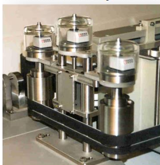
Adjustment mechanism for endless rubber masking belts
