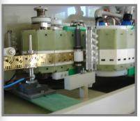
The **SPOTTER-VT** allows the plating on flat semi-conductor frames or formed contact terminals with possibilities such as spot or stripe plating on one or **simultaneously** on two sides, precise and exclusive East/West plating of **contact edges** or North/South plating by inserting silicone masking forms between the contact terminals.
