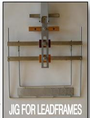
The LPP 1/U plating line is using an automatic cassette to cassette loading/unloading system. The transfer of the strips from the jigs to the SPOTTER-CS masking plates (and back to the jigs after "spot" plating) is made by an automatic "pick and place" handling mechanism.
